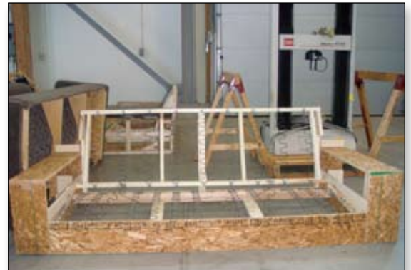
Figure 1: Typical furniture frame manufactured with OSB components.
