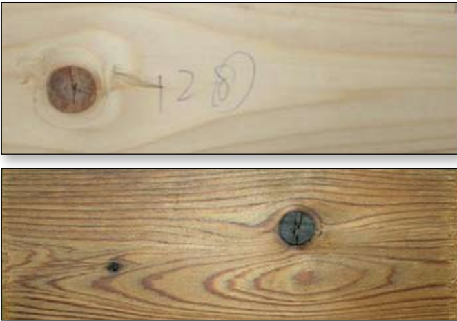
Figure 1: Colour change in pine from thermal treatment in soybean oil at 220°C for 2 hours.
