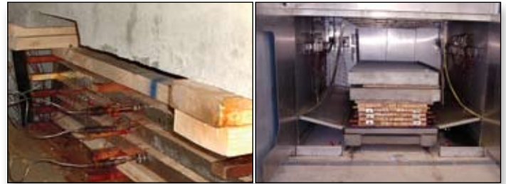
Figure 2: Experimental setup for validation tests: a) lumber stack into kiln; b) sensors to measure wood pressure and temperature.
