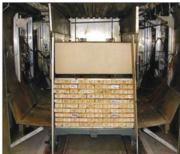
Figure 1: Load of spruce stands in experimental kiln.
