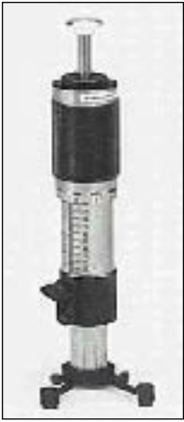
Figure 1. Handheld Impact Indenter
