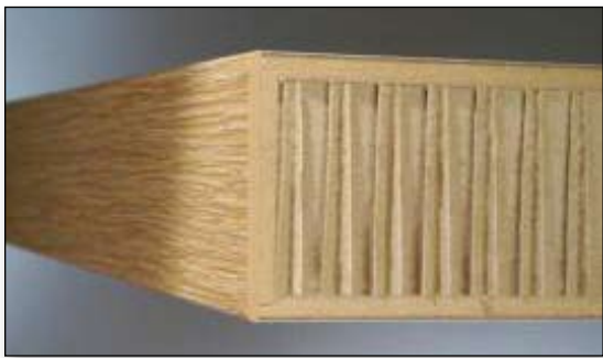
Figure 6: Direct application of an edgeband on a lightweight panel comprised of an expanded paper honeycomb core and particleboard face layers 8 mm thick ( www.doellken-kv.de ).
